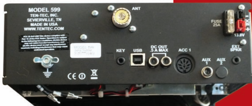
The rear panel is also of simple layout. Note though, the unusual power socket and vehicle style fuse on the upper right corner.
