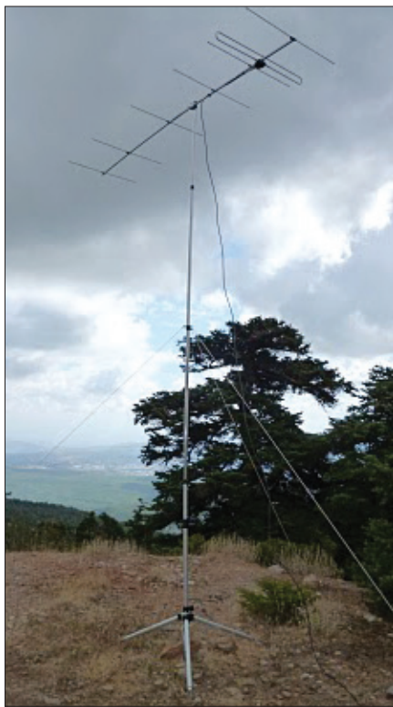
A 7-element Yagi antenna standing on a portable tripod mount and supported by guy ropes - from the Greek side of Panis' contacts.
