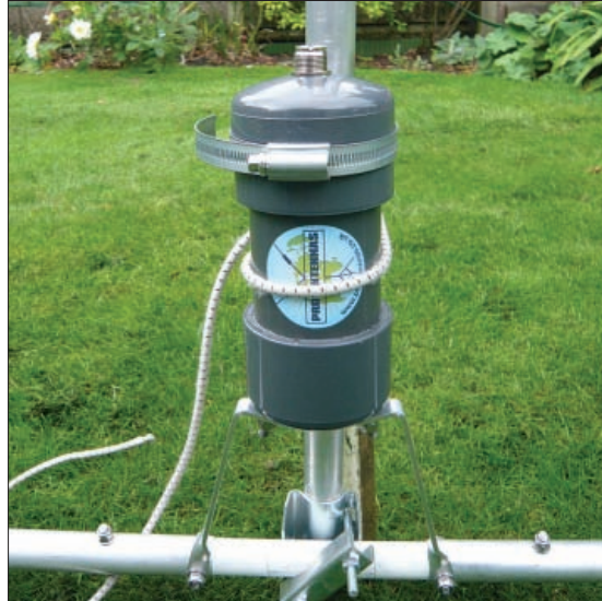
A close-up of the 'potted' balun.
