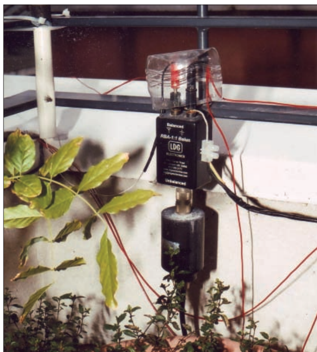
Fig. 3: The LDG 1:1 balun used by Jonathan M5AEO. The bottom of the antenna can be seen on the left, fixed to the railings with cable-ties.
